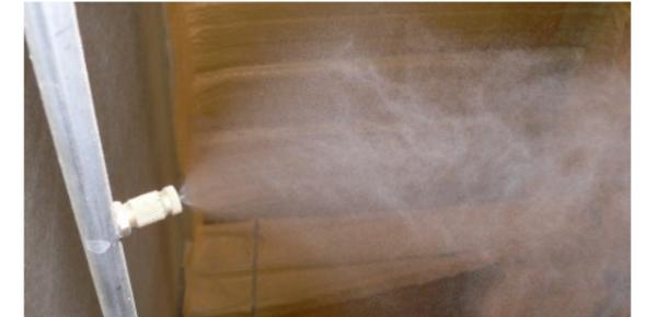
**ENG** Combined with static or dynamic ventilation, the FOGGING is the most economical system to remove the negative impact of high temperatures on production. Effective mist-spraying has to refresh without wetting. Therefore, our NOZZELS are designed to get as small droplets which guarantee their suspension in the air and the perfect interchange of coldness with the atmosphere. No dripping or moisture concentrations.
